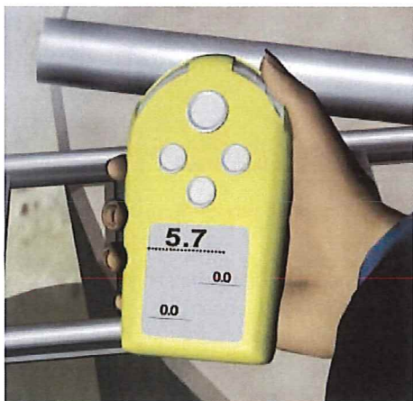
Example of a combustible gas detector used to test for the presence of flammable gas or vapor.
